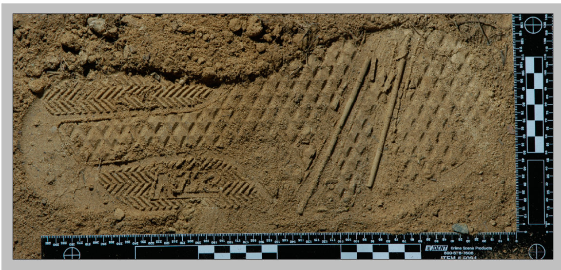
Figure 11. The cropped composite image provides a seamless, high resolution image that is better for image analysis and identification.
