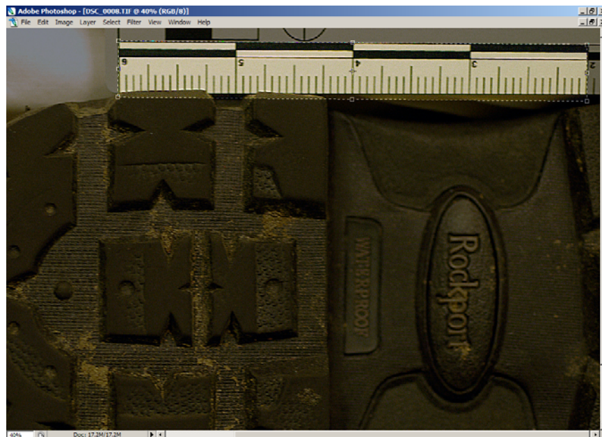
Figure 1. Using the crop tool, you can identify a specific distance within an image, which is essential for calibrating images.
