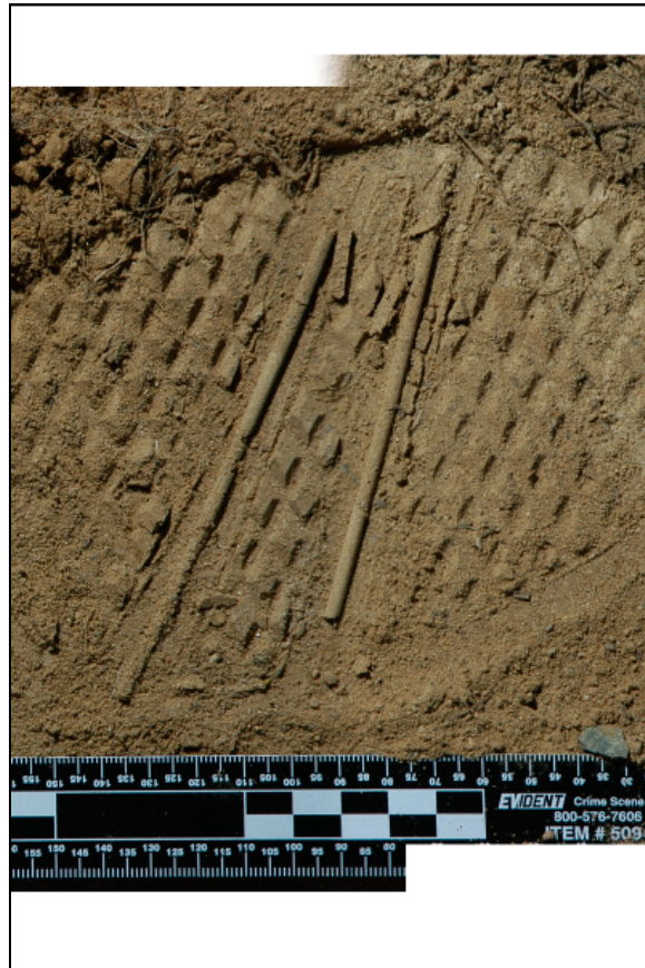
Figure 9. The feathered edge of the top (overlying) image makes the blending of the two, high resolution images appear seamless.
